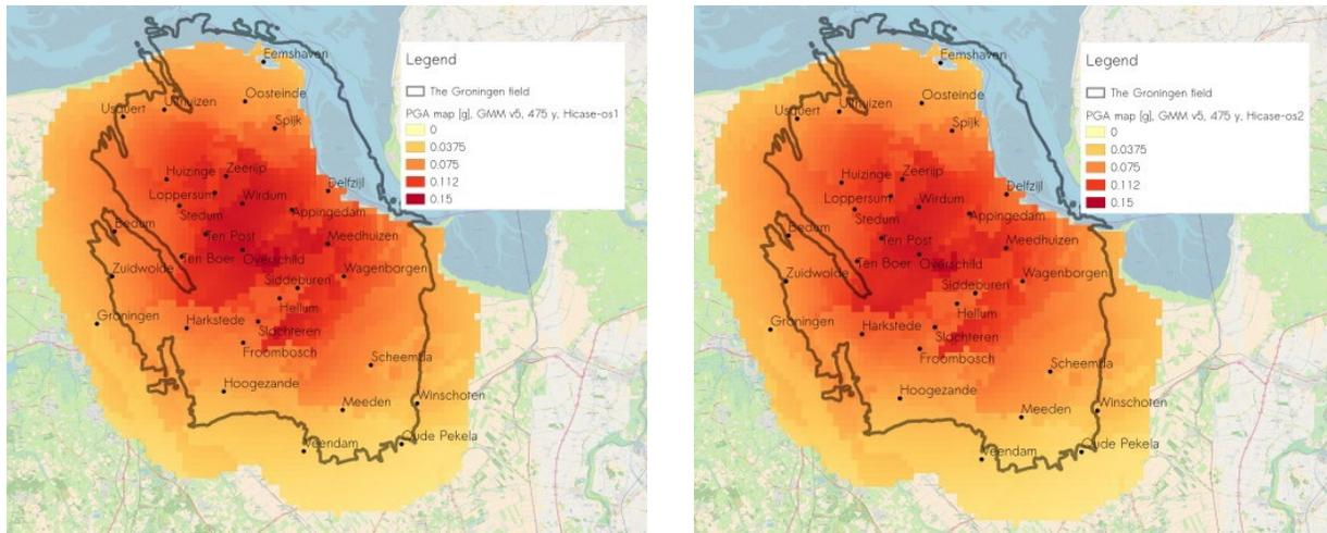
Figure 10: PGA map for Groningen for the period  $T = 0.01$  s for GMM v5 and the two production strategies for a cold winter. The return period is 475 y according to Eurocode 8. The maximum PGA is 0.14g in both maps. The black solid line indicates the boundary of the Groningen gas field.
