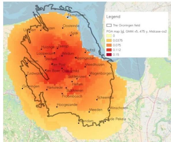
Figure 9: PGA map for Groningen for the period  $T = 0.01$  s for GMM v5 and the two production strategies for an average winter. The return period is 475 y according to Eurocode 8. The maximum PGA is 0.14g and 0.13g, respectively. The black solid line indicates the boundary of the Groningen gas field.
