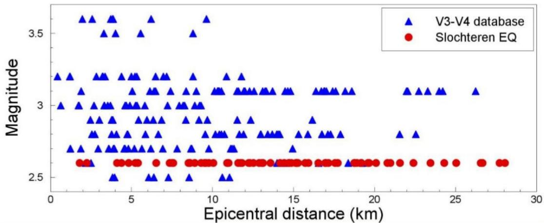
Figure 6: The event data base used in the construction GMM V5. (The GMM v5 report by Bommer et al., 2018).
