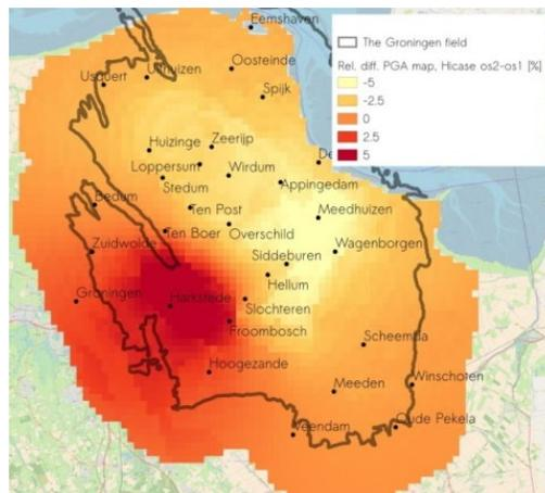
Figure 11: Difference between the PGA maps for the two operational strategies for the warm, average and cold winter scenario in Figure 10. The black solid line indicates the boundary of the Groningen gas field. PGA differences are indicated in %.
