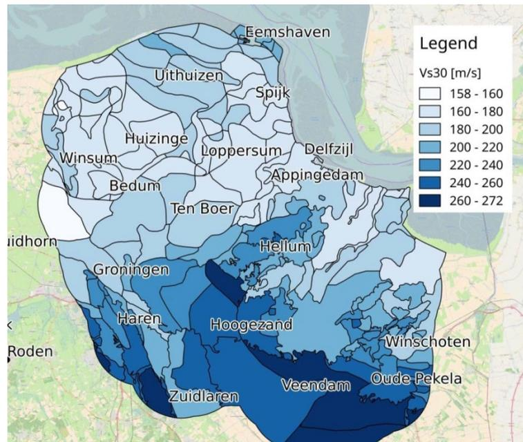
Figure 7: Geological zones and shear wave velocities in the shallow subsurface (Kruiver et al., 2017).
