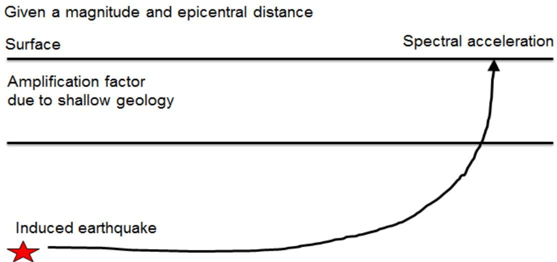
Figure 5: Schematics of the two-layer model used to define the GMM v2 to v5.
