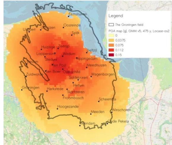
Figure 8: PGA map for Groningen for the period  $T = 0.01$  s for GMM v5 and the two production strategies for a warm winter. The return period is 475 y according to Eurocode 8. The maximum PGA is 0.13g in both maps. The black solid line indicates the boundary of the Groningen gas field.
